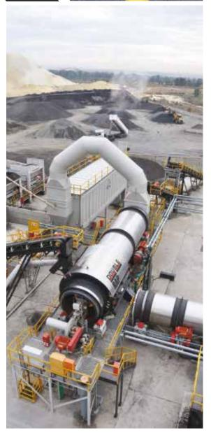
Double barrel RA twin drum with foaming capabilities (located at Much Asphalt Benoni)
